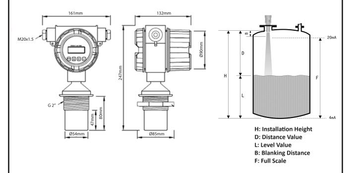
The meter measures time t between pulse transmission and reception, uses time t (and the velocity of sound c) to calculate distance D between sensor membrane and product surface: D = c •t/2. With pre-setting empty distance H, level value then be calculated: L = H - D
