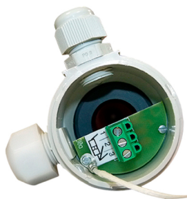
Connector to built-in Pt 100 sensor
