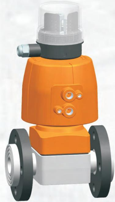
MV303 is a type of standard chemical grade pneumatic diaphragm valve, which has the new design of smooth runner for superior performance for big flow and the overall mechanical mechanism is more optimized. This type of valves has high performance applications for water and chemical with PN10 pressure rate.
